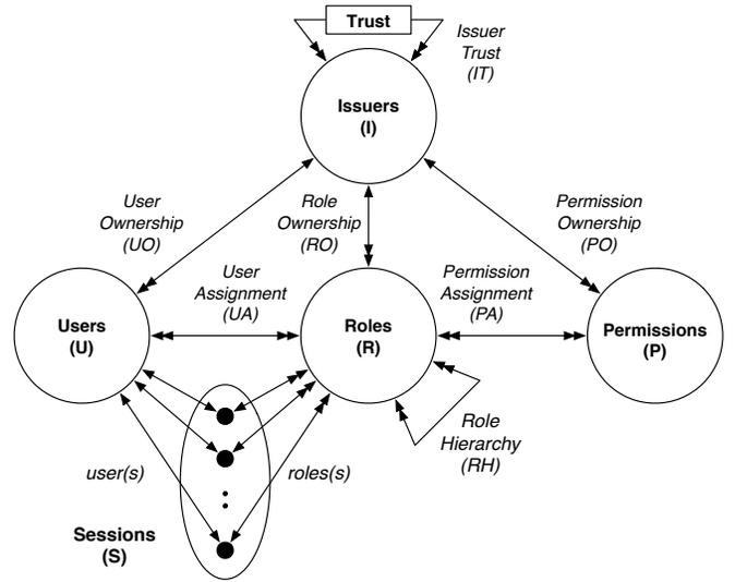
Figure 2. An abstracted model of the MTAS system.
