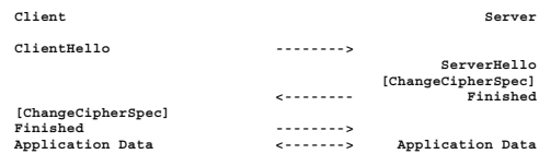
Fig. 2 - Message flow for an abbreviated handshake
